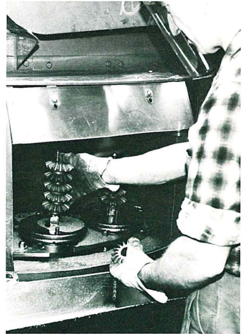
Operator loads five gears on spindle fixture on one of the work tables of the seven machines installed at Ford for shot peening.
